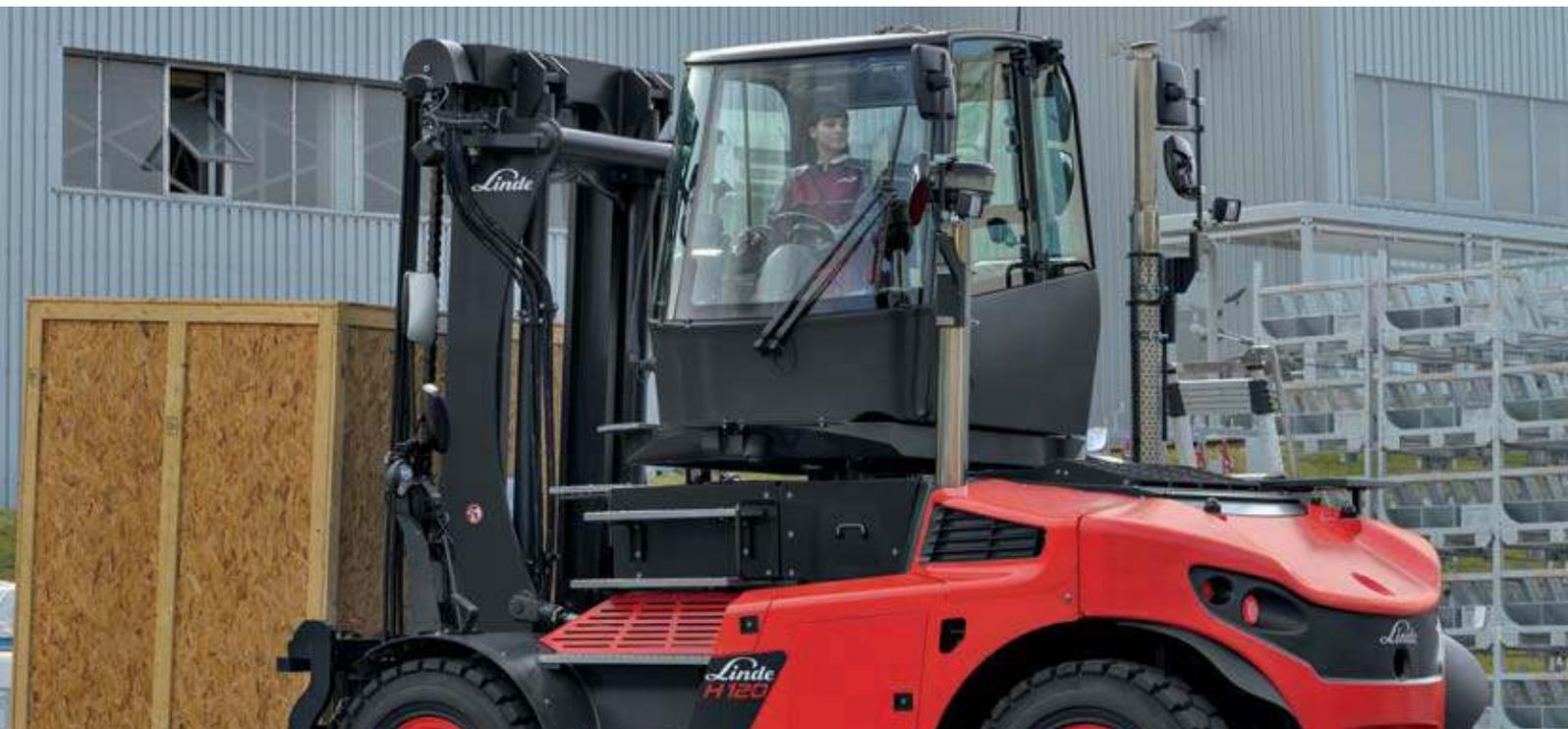
With the help of the rotating cab, the driver always has an optimum circumferential view. Compared to the standard model, the cab height is increased by 600 millimetres, and the cab can be rotated in infinitely variable stages using the joystick or the position switches by up to 180 degrees to the left or 65 degrees to the right.
